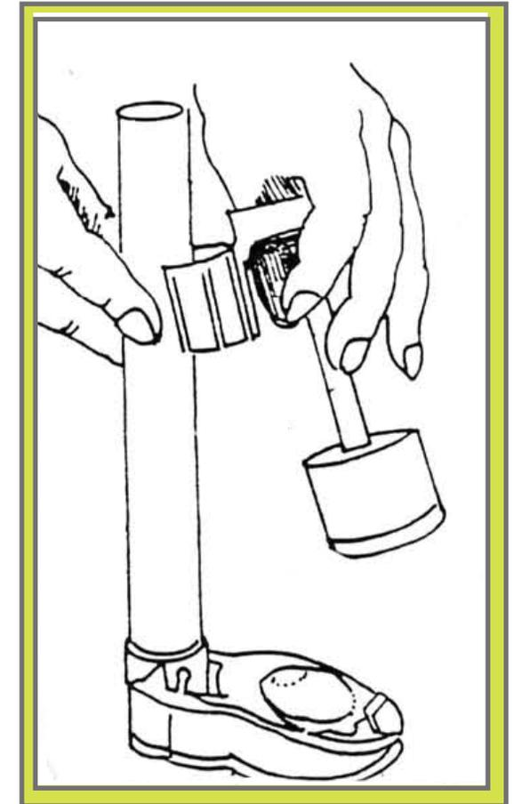
The watersaver Pop Flush is an early flapper closure device. This ingenious little product is an inexpensive alternative to replacing your high consumption toilet. Savings range from 1.5 to 3 gal./flush.
